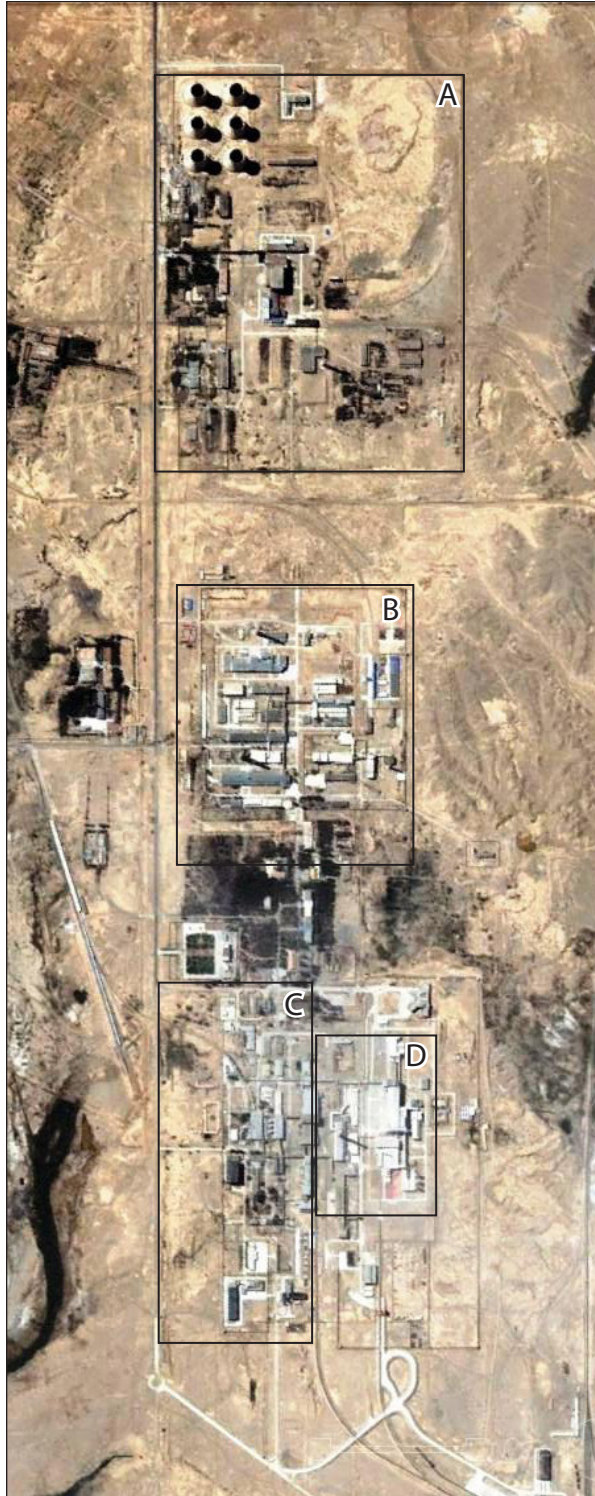
Overview of Jiuquan Nuclear Complex: Box A shows the complex's reactor area; Box B shows the intermediate pilot reprocessing plant; Box C shows the military reprocessing plant; Box D shows the civilian pilot reprocessing plant. (Source: DigitalGlobe and Google Earth, Aug. 31, 2007.)
