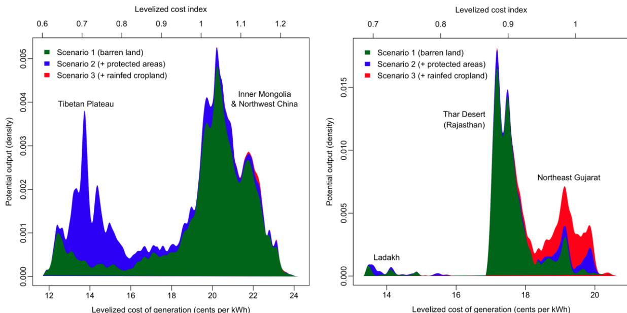
The levelized cost estimates presented throughout this paper assume that CSP construction costs do not differ across locales; that is, differences in the LCOE index are determined solely by the modeled relationship between solar radiation, latitude, and plant efficiency. In practice, some locales will face site-specific conditions (lack of transport access or nearby labor supply, for example) that impact costs and are not captured here.
