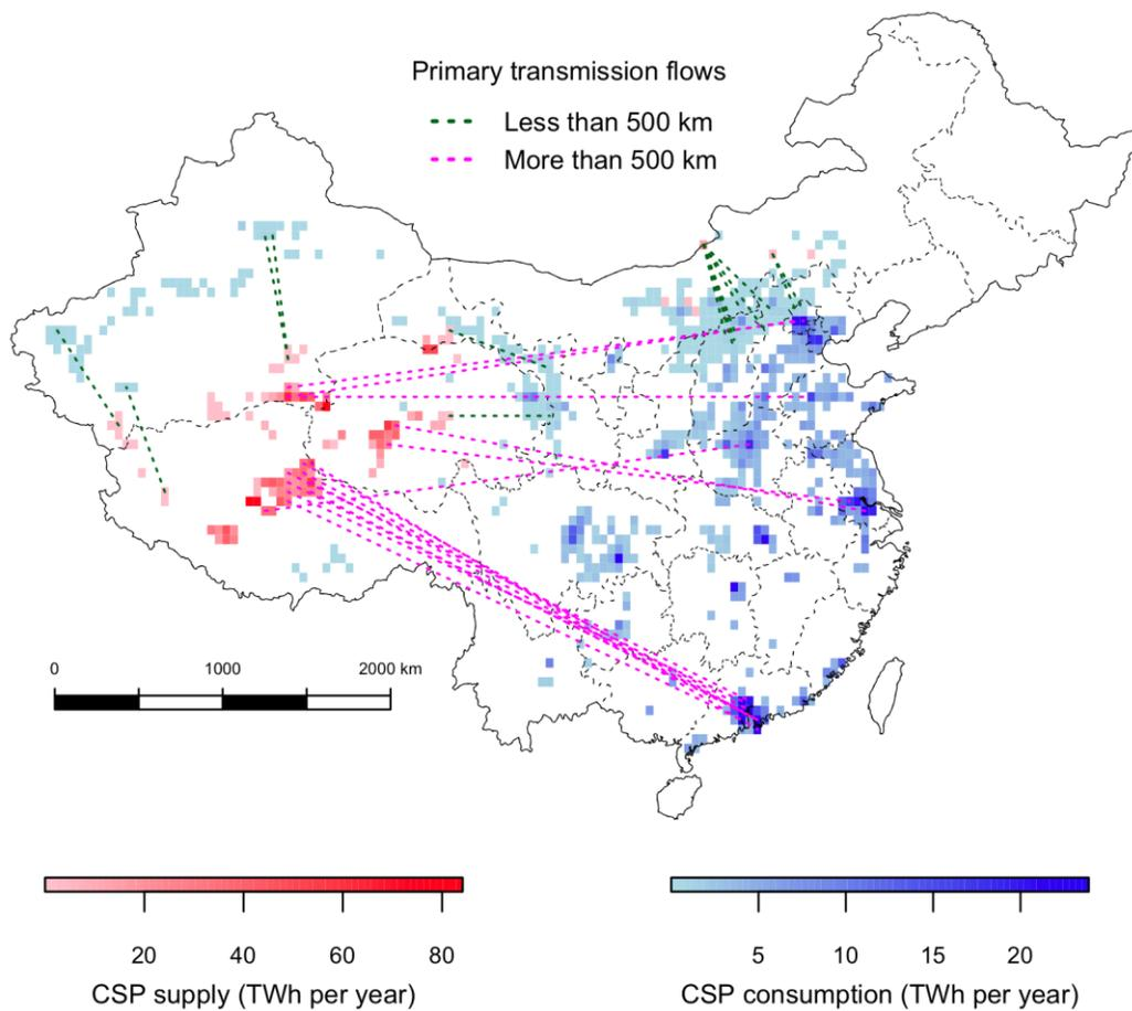
The results for China reveal concentration of generation on the Tibetan Plateau, where higher efficiencies and lower generating costs offset the additional cost of transmission to eastern cities. Three primary, long-distance transmission flows bring power from the plateau to the Hong Kong, Shanghai, and Beijing areas.
