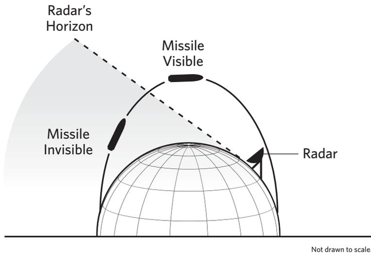
The trajectory of a ballistic missile with a range of 3,500 km and the horizon of a powerful early warning radar located 500 km (310 mi.) forward of the impact point are shown
