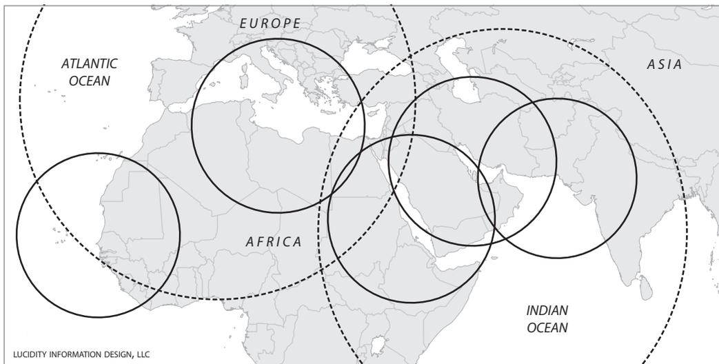
The solid and dashed lines show the coverage of, respectively, five ships or submarines carrying hypersonic cruise missiles with a range of 1,500 km, and two vessels carrying ballistic missiles with a range of 3,500 km (firing positions about 100 km from the nearest coast are assumed). Alternatively, a single deployment of boost-glide weapons based on the Advanced Hypersonic Weapon could provide complete coverage of the region.
