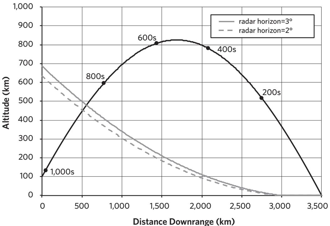
The missile is travelling from left to right and the time until impact is shown in increments of 200 secs. The radar is located 500 km in front of the missile’s impact point. Author calculation.
