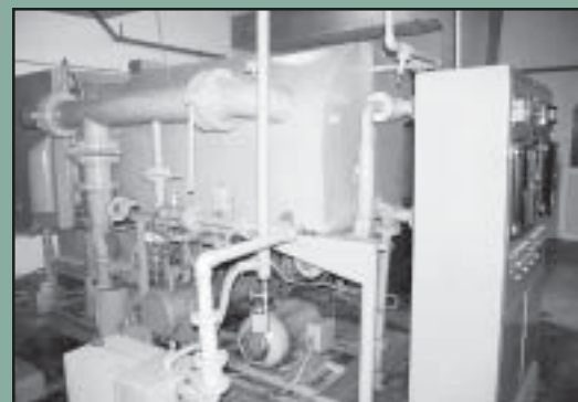
From top: entrance gate at LABIOFAM; Terence Taylor swipes in with his magnetic card at LABIOFAM gate; Gen. Wilhelm inspects the vaccine freeze dryer at LABIOFAM; the freeze dryer was reported to have a capacity of 180 liters per 24 hours.
