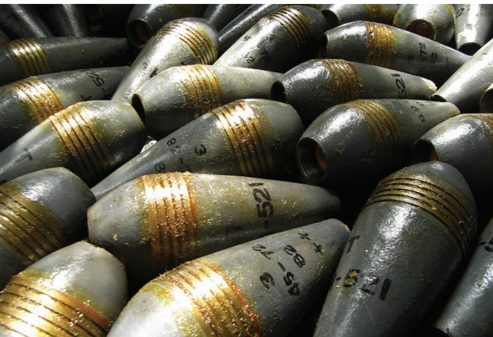
60 mm mortar ammunition scrap following melting operation, Albania. © NAMSA
