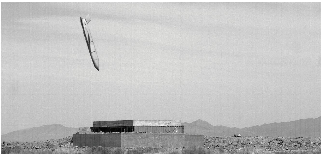
Joint Air-to-Surface Stand-off Missile (JASSM) moments before penetration into test target. Photo: Lockheed Martin Corporation. Copyright 2012.
