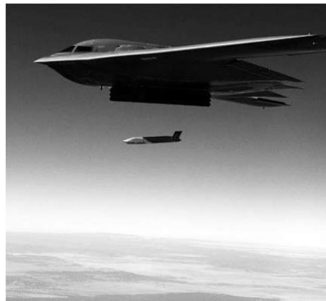
The AGM-158 JASSM, an air-to-ground missile designed for Air Force and Navy jet fighters, is pictured above being launched by a B-2 Spirit bomber.
