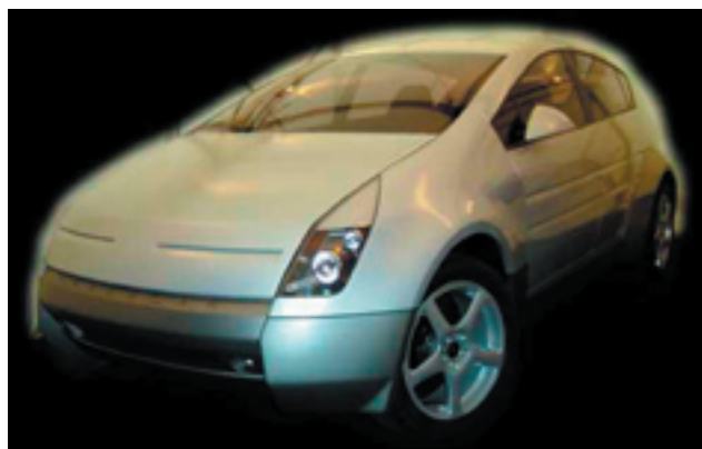
Figure 1: The Revolution concept car, an ultralight (857-kilogram) carbon-fiber mid-size sport utility vehicle, designed in 2000.
