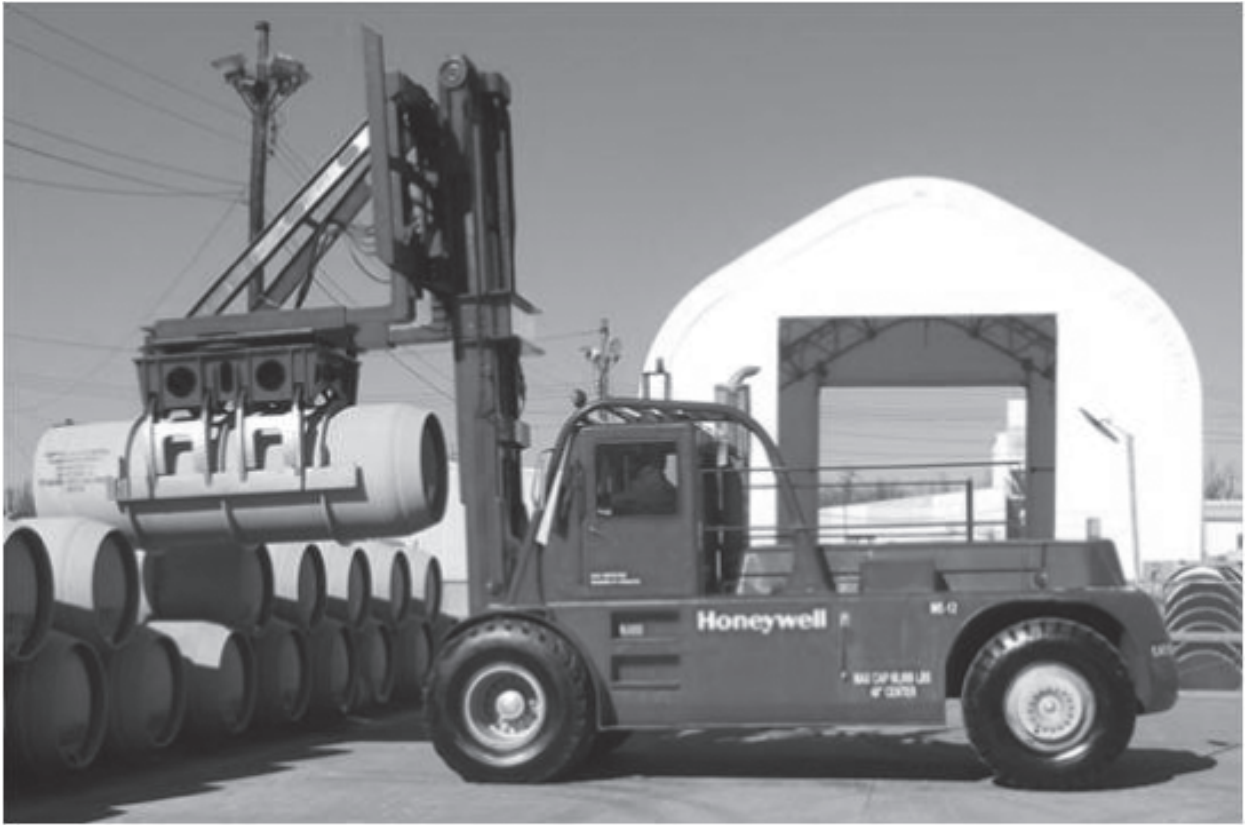
Uranium hexafluoride ( UF_6 ) Type 48Y cylinder being moved at Honeywell Metropolis Works, Metropolis, Illinois. Source: Wikipedia. http://en.wikipedia.org/wiki/File:Cylinder_Load.jpg .
